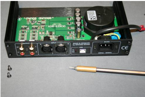
Fix the Sides to BackPanel with M4x10mm
