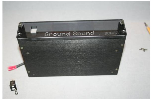
Mount Front Panel – don't use excessive force
