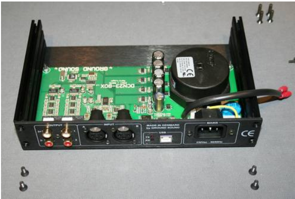
Glide Sides onto nuts on Bottom Plate
