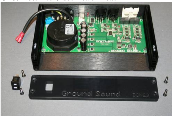
Prepare Front Panel/Switch/M4x16mm
