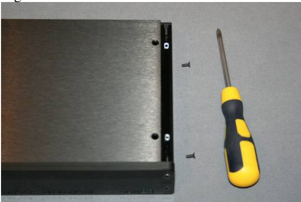
Adjust distance of nuts and mount M3x8 screws
