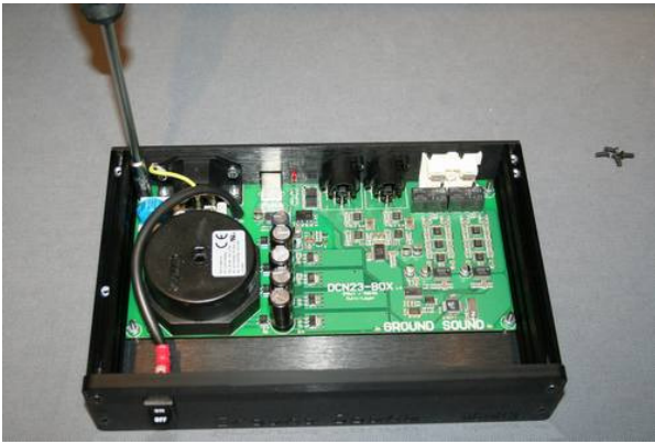
Tighten nuts on PCB
