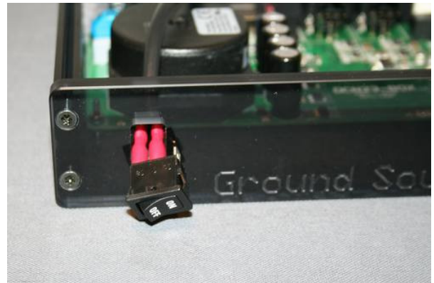
Assemble cable and Power Switch
