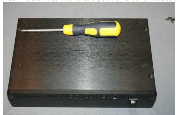
Tighten screws on the bottom
