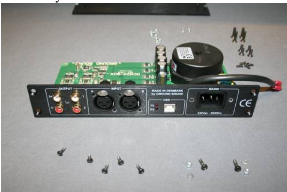
Assembly of Back Panel on PCB Screw 2,9x9
