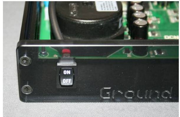
Push Power into FrontPanel, some force is needed
