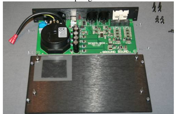
Mount PCB/BackPanel on Bottom Plate
